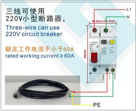
Depending on the power of the laser, below 2KW: using 220V single-phase three-wire power cords, circuit breakers with a rated working current ≥60A; 2KW and above: using 4-
